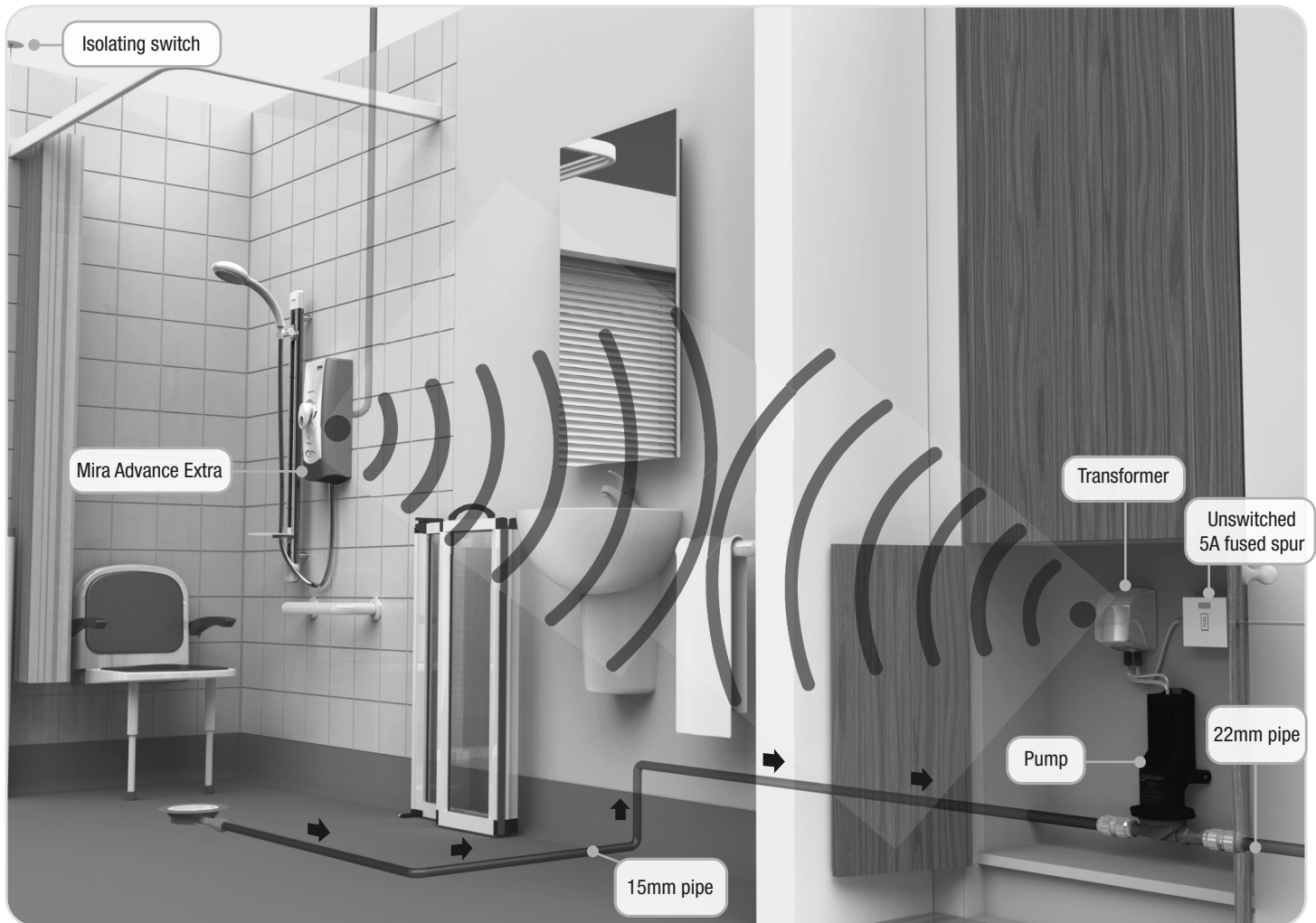
Range = 5 metres maximum for wireless signal Typical INSTANT MATCH wireless wet floor installation
